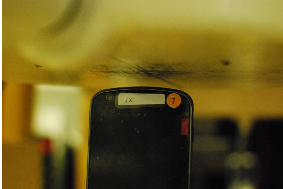
SAR Test Setup Photo 7: Top at 1.0cm
