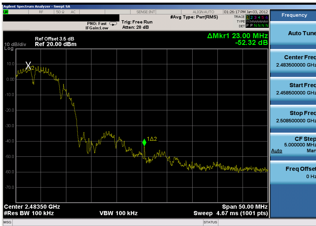
Plot 6-20. Band Edge Plot (802.11b – Ch. 11)
