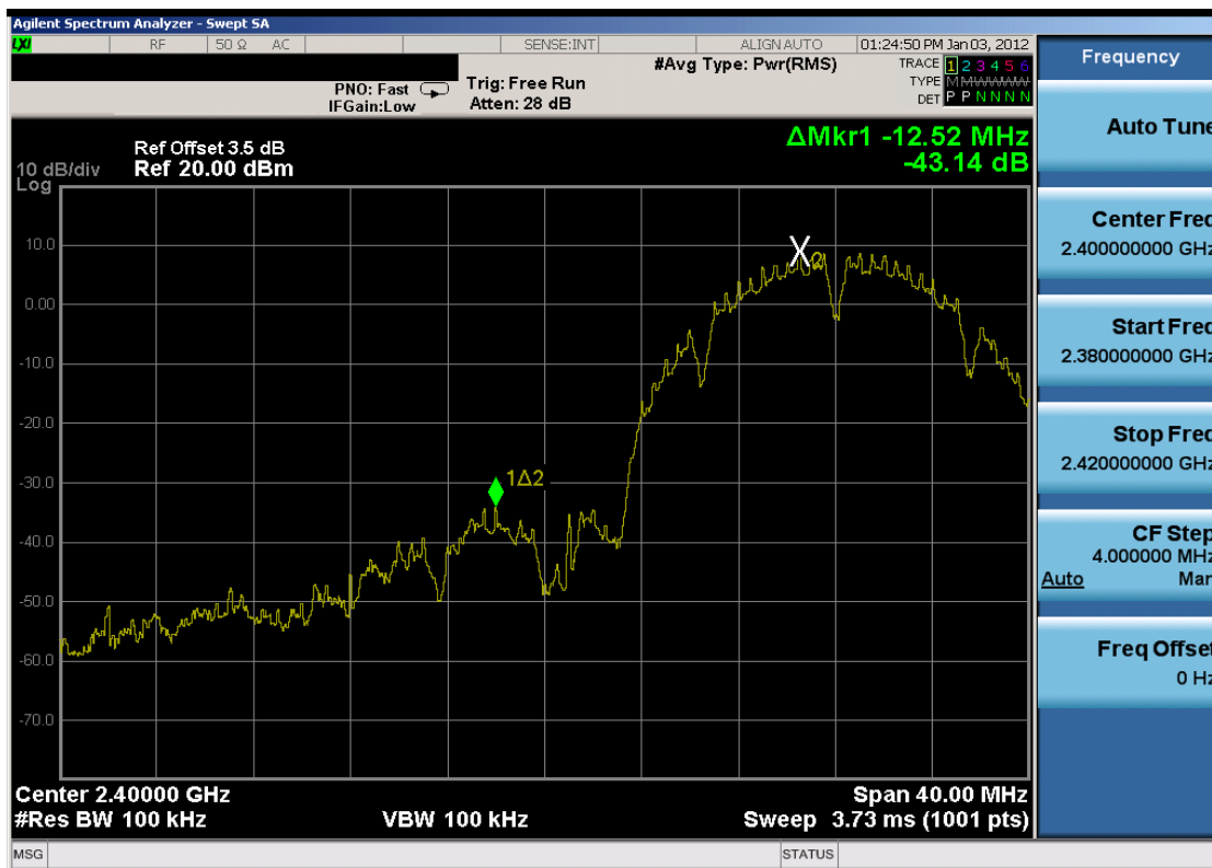
Plot 6-19. Band Edge Plot (802.11b – Ch. 1)
