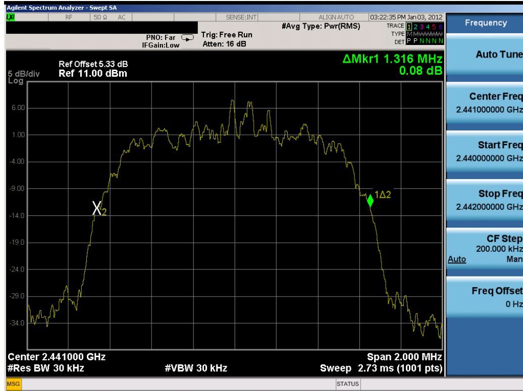
Plot 6-5. 20dB Bandwidth Plot (Bluetooth, 2Mbps - Ch. 39)
