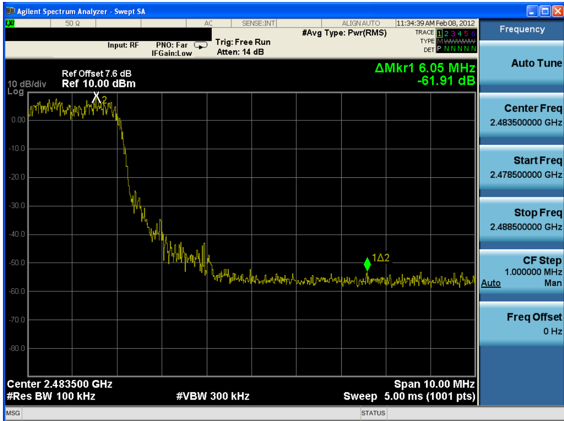
Plot 6-13. Band Edge Plot (Bluetooth with Hopping Enabled, 2Mbps – Ch. 78)
