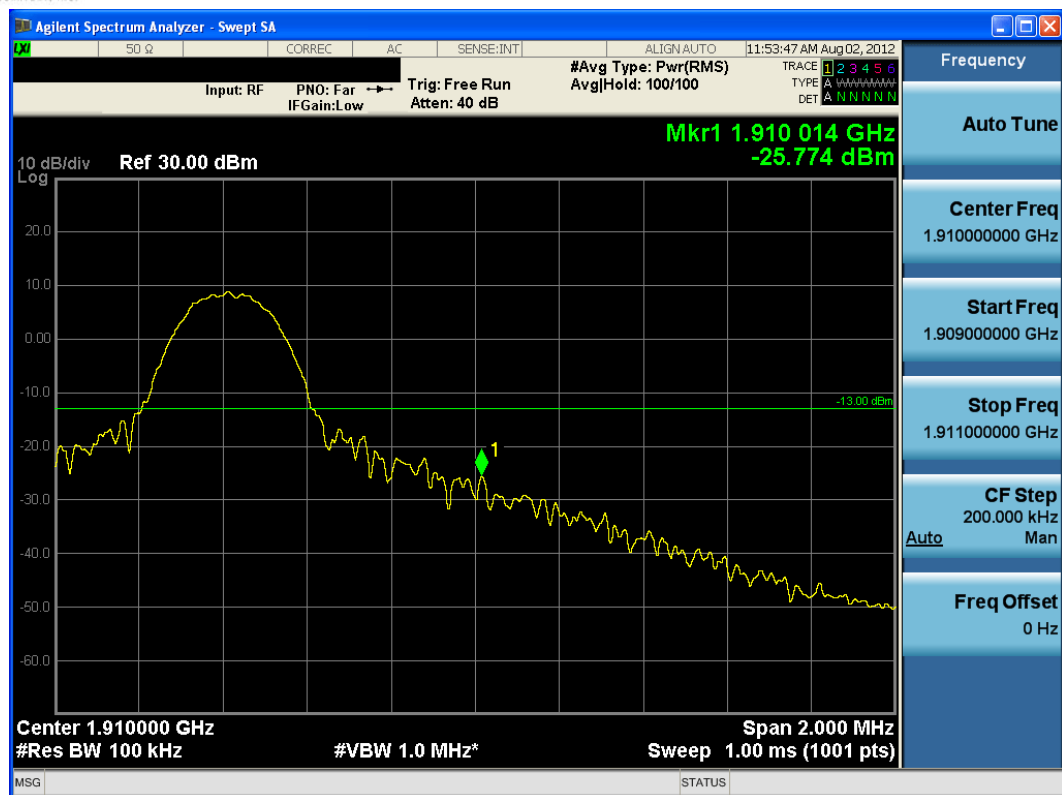
Plot 7-22. Upper Band Edge Plot (QPSK – RB Size 1, RB Offset 0)
