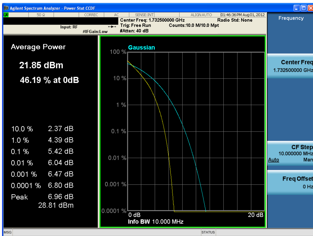
Plot 7-4. Peak to Average Ratio Plot (QPSK - RB Size 50)
