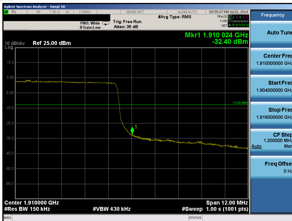
Plot 6-31. Upper Band Edge Plot (Band 2 - 15.0MHz QPSK - RB Size 75)
