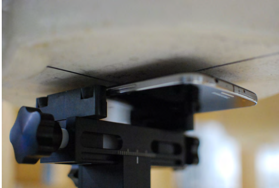
SAR Test Setup Photo 5: Back Side at 1.0 cm
