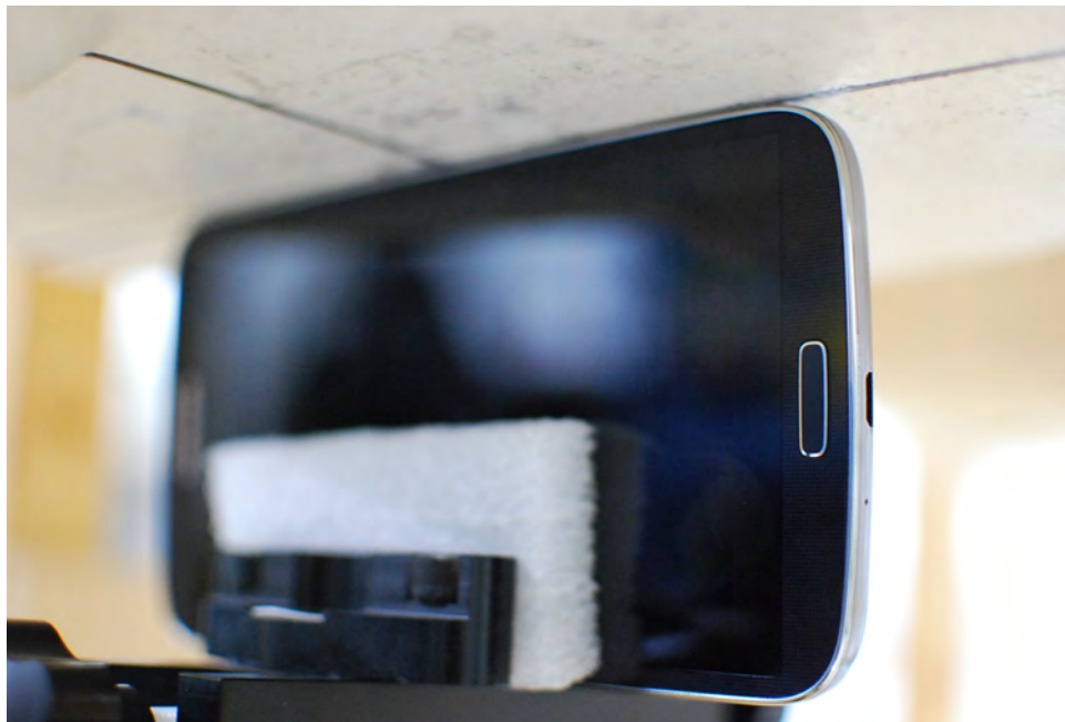
SAR Test Setup Photo 12: Right Edge at 0.0 cm
