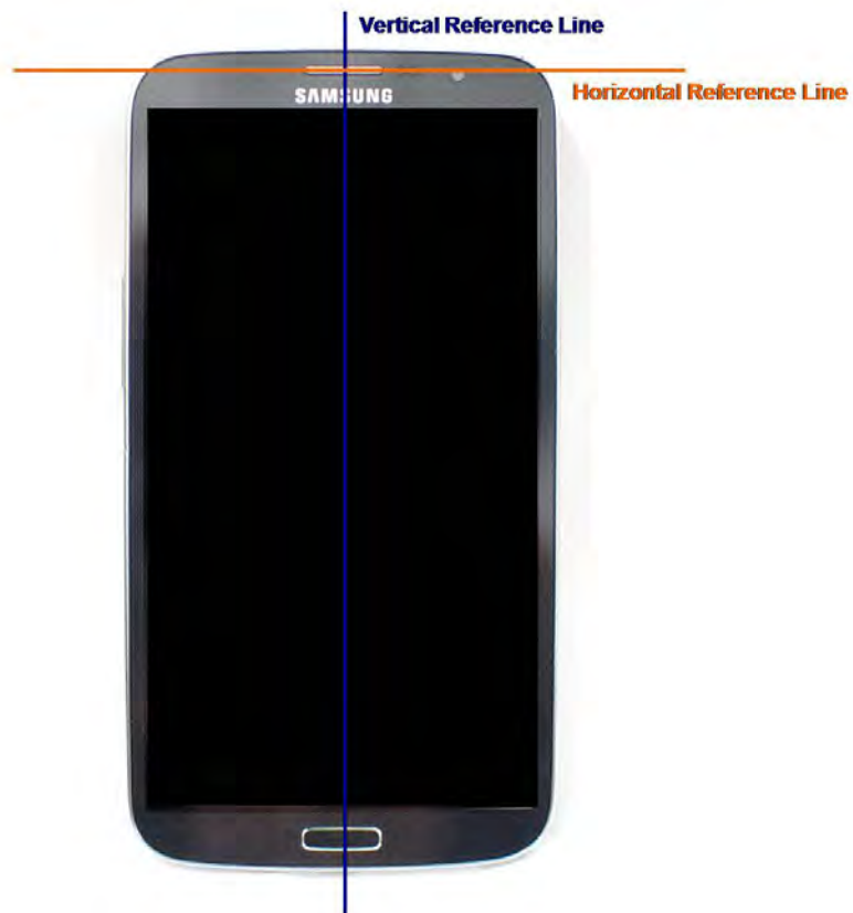
SAR Test Setup Photo 14: Horizontal and Vertical Reference Lines
