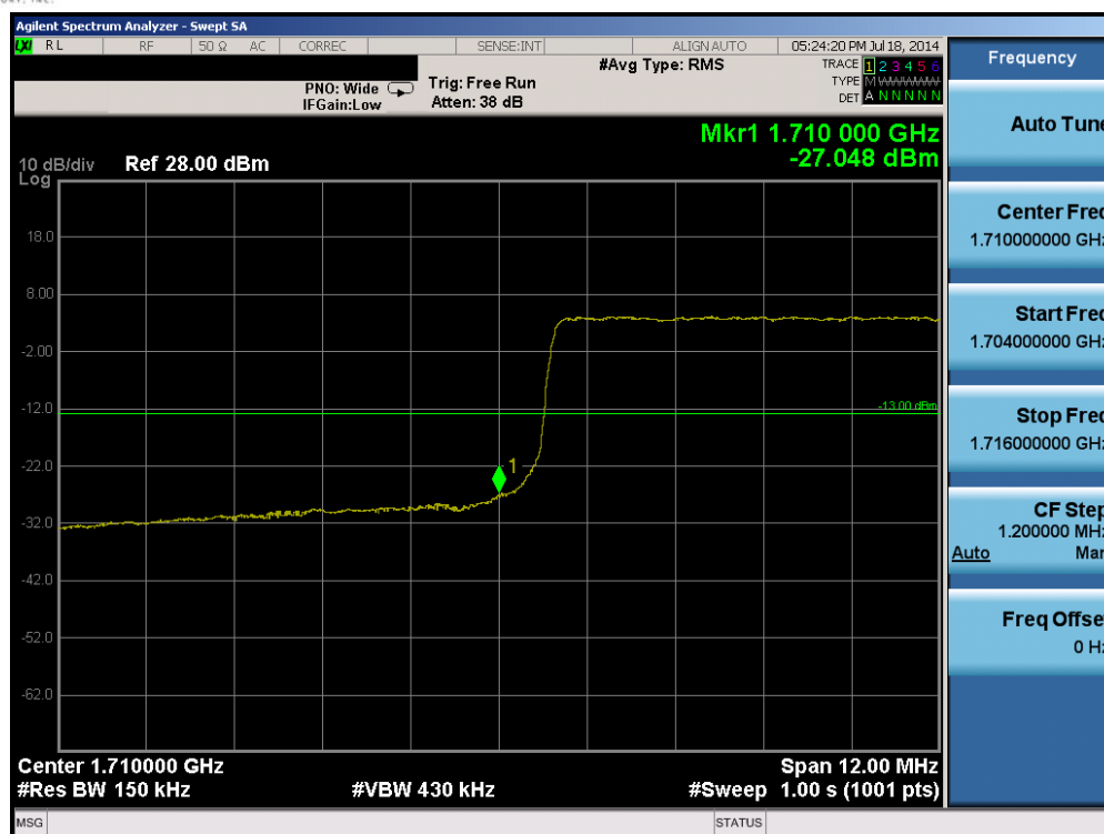
Plot 6-21. Lower Band Edge Plot (Band 4 – 15.0MHz QPSK – RB Size 75)
