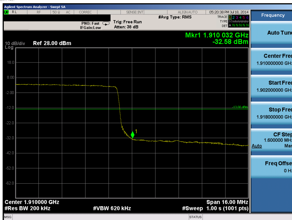
Plot 6-35. Upper Band Edge Plot (Band 2 – 20.0MHz QPSK – RB Size 100)
