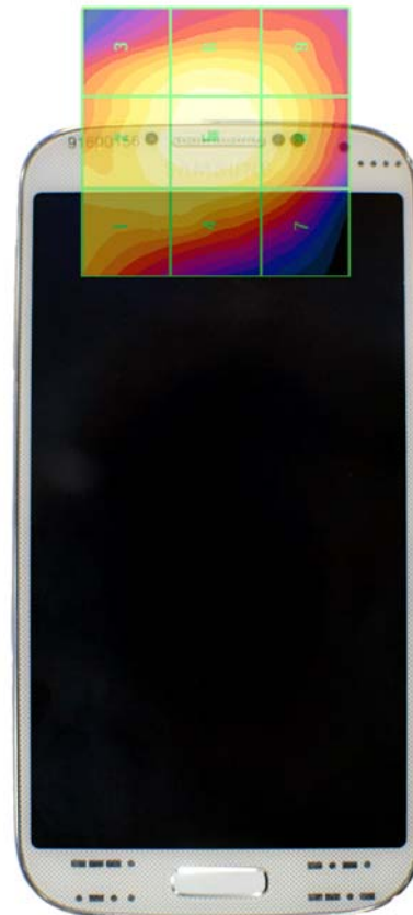
Figure 17-5 H-Field WD Scan overlay
