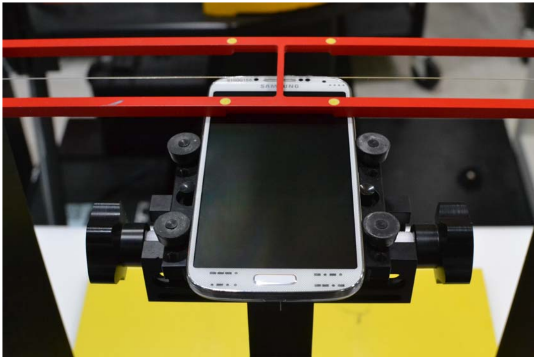
Figure 17-2 HAC Phantom Plane Alignment
