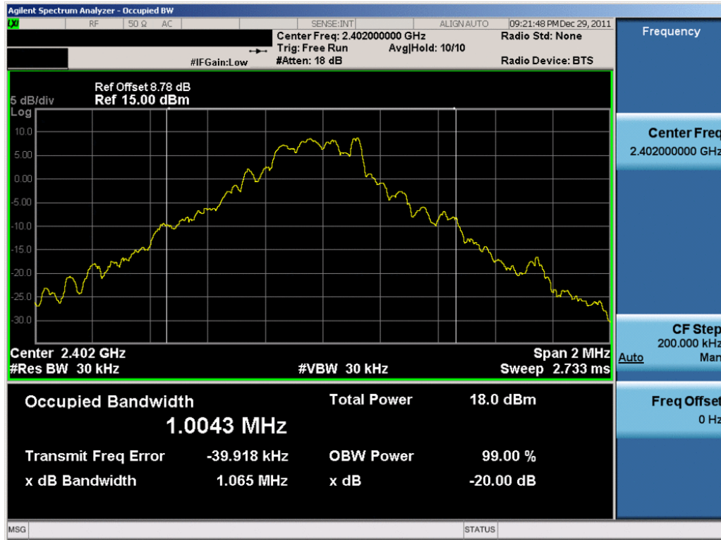
Plot 6-1. 20dB Bandwidth Plot (Bluetooth, 1Mbps – Ch. 0)
