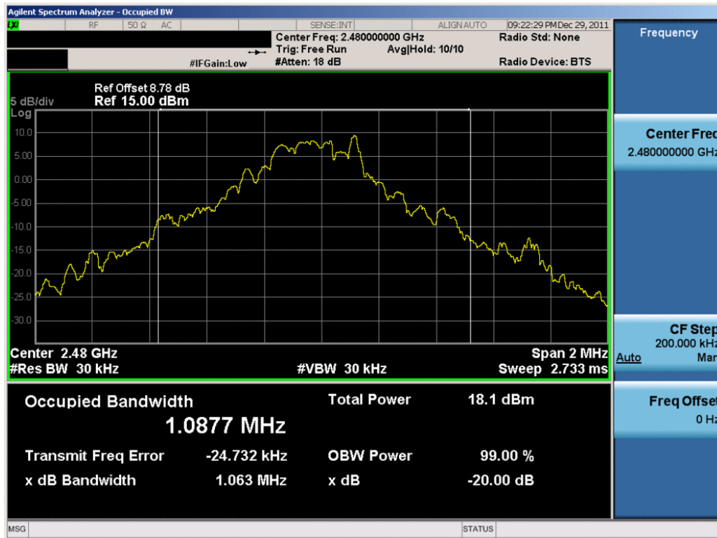
Plot 6-3. 20dB Bandwidth Plot (Bluetooth, 1Mbps – Ch. 78)
