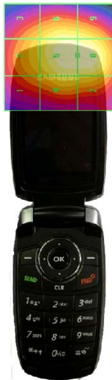
Figure 17-4 E-Field WD Scan overlay
