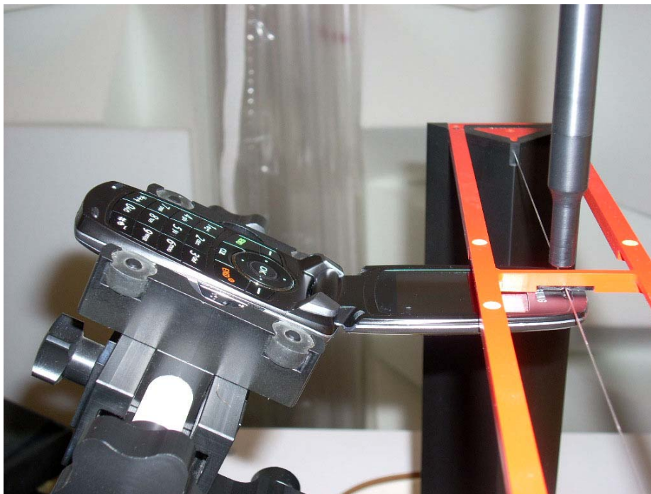
Figure 17-1 Ear Reference Point HAC Phantom Alignment
