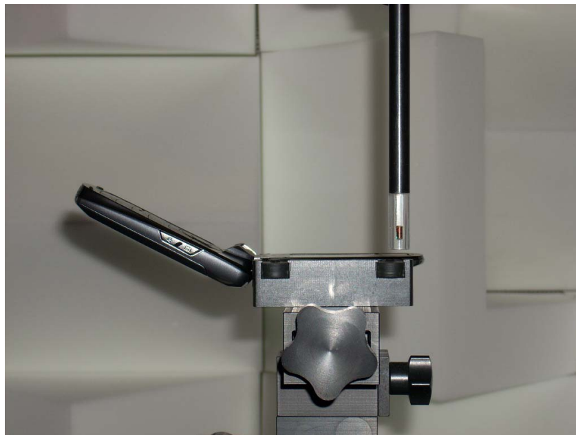
Figure 13-2 Test Setup for Wireless Device
