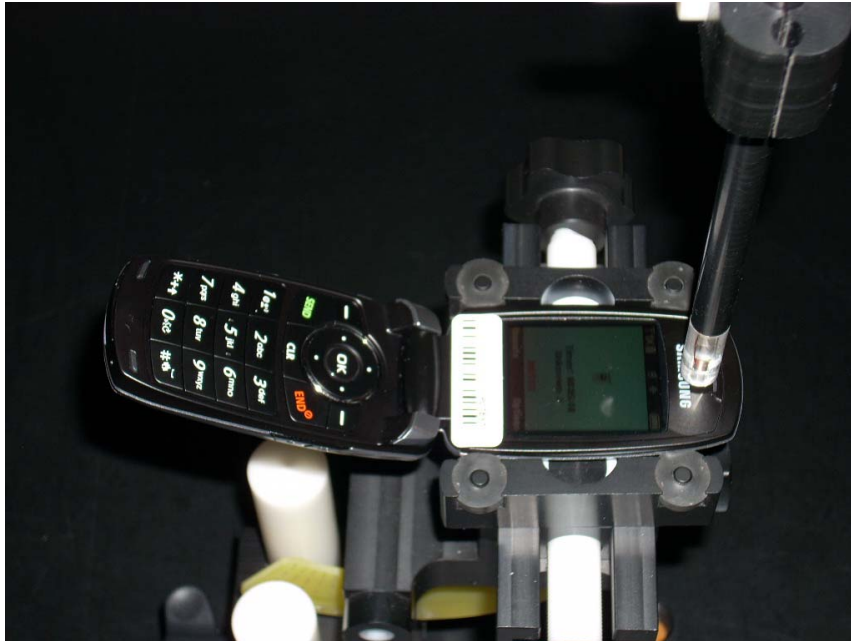
Figure 13-1 Test Setup for Wireless Device
