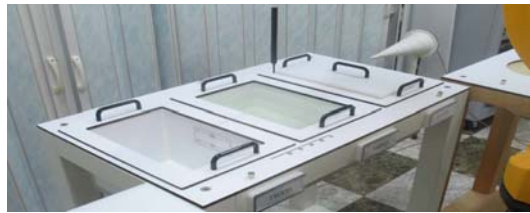
Figure 3.6 Modular Flat Phantom
