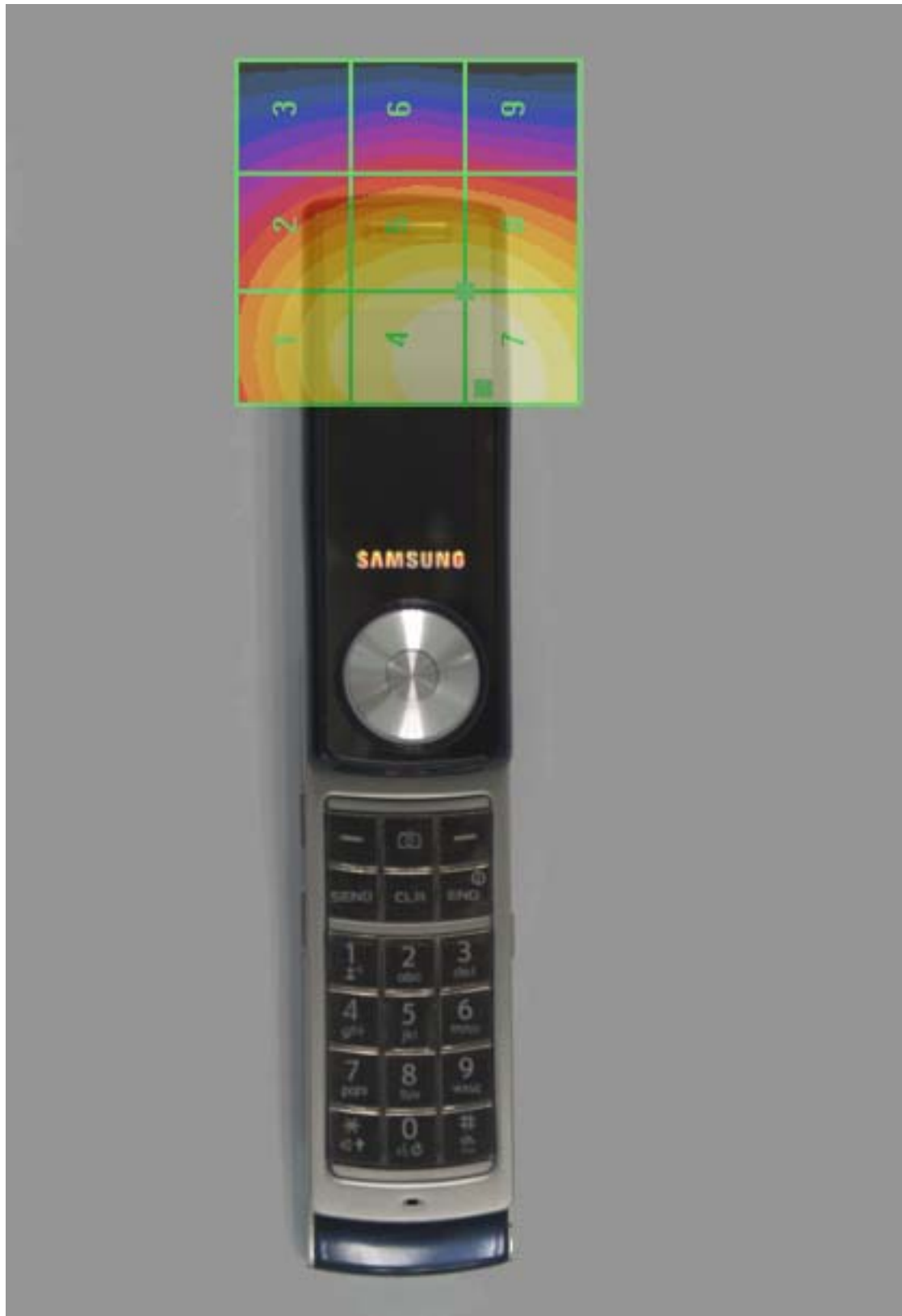
H-Field scan overlay with actual device
