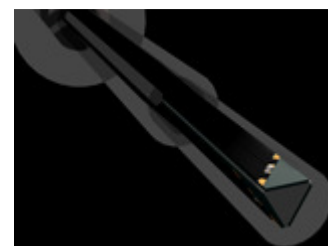
Figure 4-3 Triangular Probe Configuration
