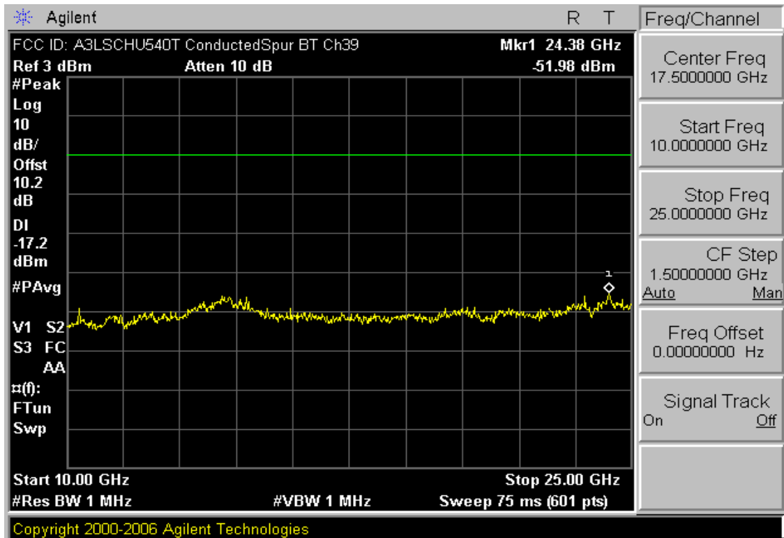
Plot 6-13. Conducted Spurious Plot (Bluetooth – Ch. 39)
