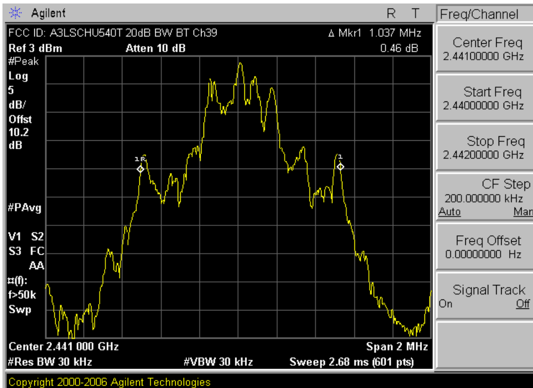
Plot 6-2. 20dB Bandwidth Plot (Bluetooth – Ch. 39)
