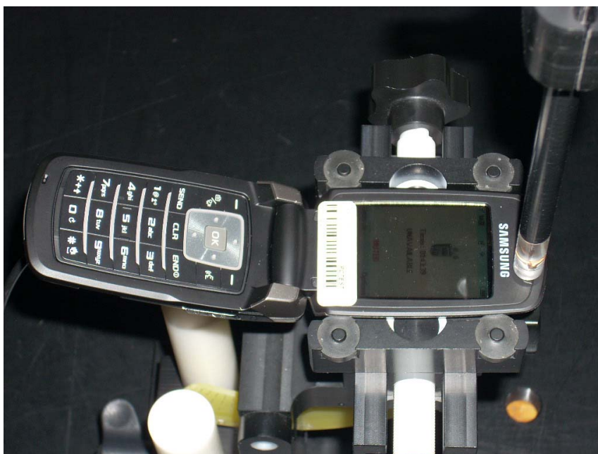
Figure 13-1 Test Setup for Wireless Device
