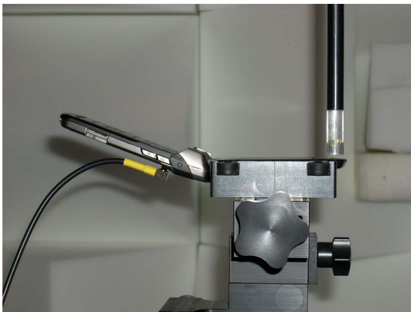
Figure 13-2 Test Setup for Wireless Device
