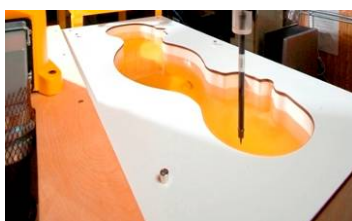
Figure 6-2 SAM Phantom with Simulating Tissue
