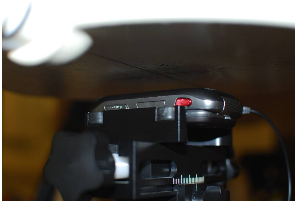
Figure 19-6 SAR Test Setup Photo 6 – Body, 1.5 cm spacing
