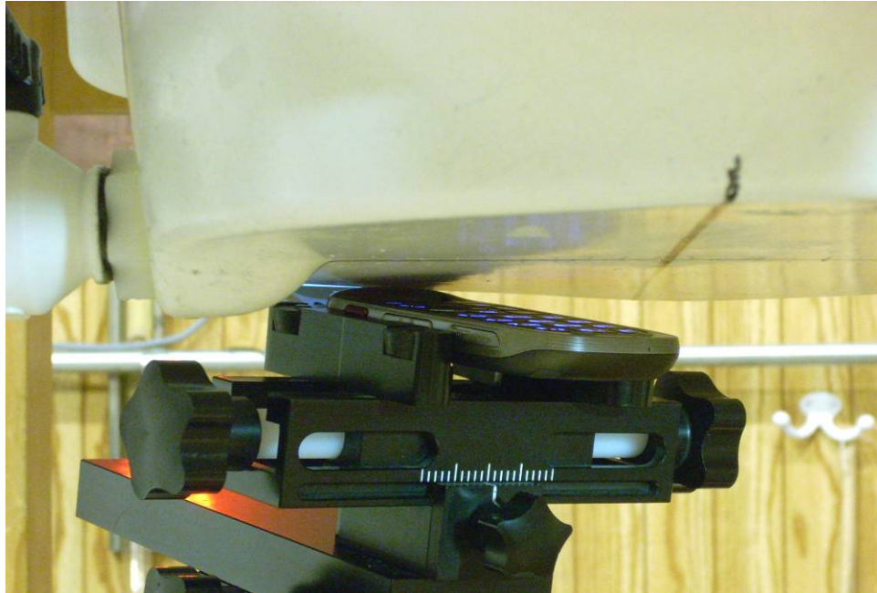
Figure 19-1 SAR Test Setup Photo 1 – Mouth-Jaw 1.8 cm
