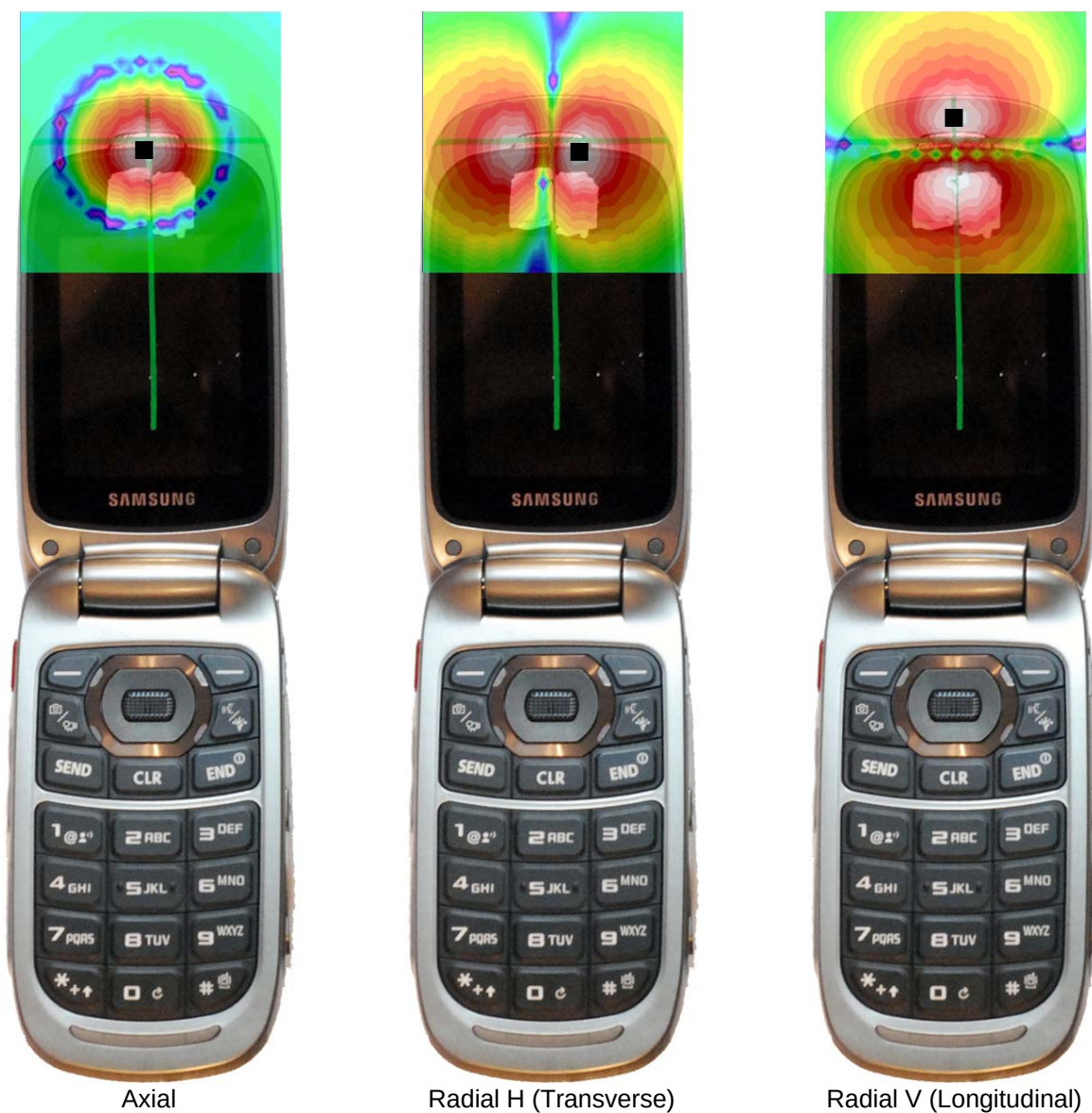
Figure 13-3 T-Coil Scan Overlay Magnetic Field Distributions
