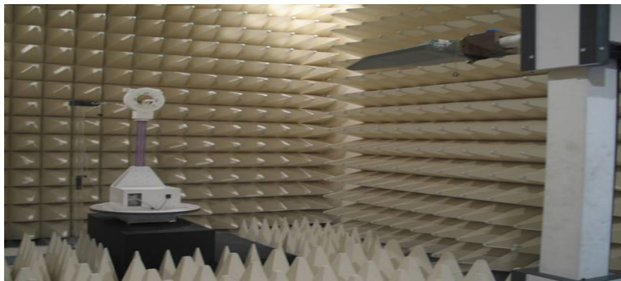
Figure2. Photograph of 3m Fully-Anechoic Chamber
