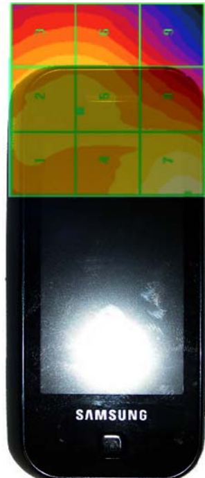
Figure 17-5 H-Field WD Scan overlay
