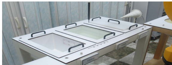
Figure 3.6 Modular Flat Phantom
