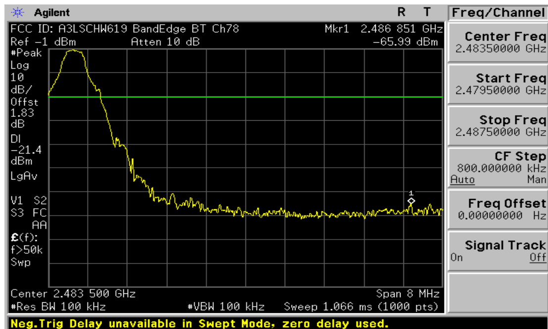
Plot 6-5. Band Edge Plot (Bluetooth – Ch. 78)
