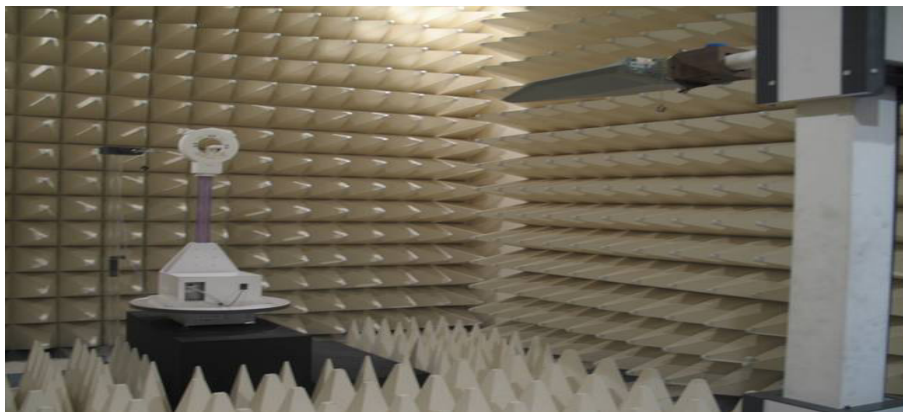
Figure2. Photograph of 3m Fully-Anechoic Chamber
