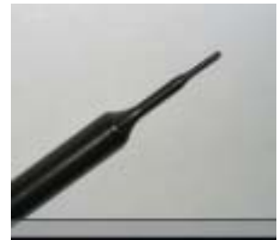
Figure 3.4 Probe Thick-Film Technique
