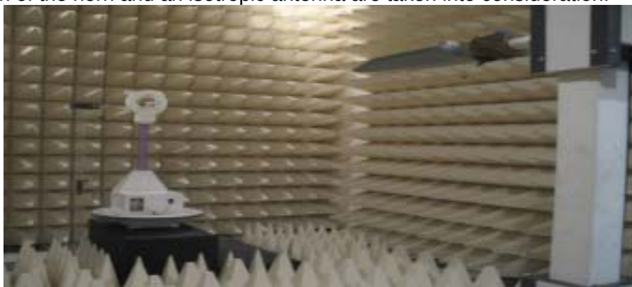
Figure2. Photograph of 3m Fully-Anechoic Chamber
