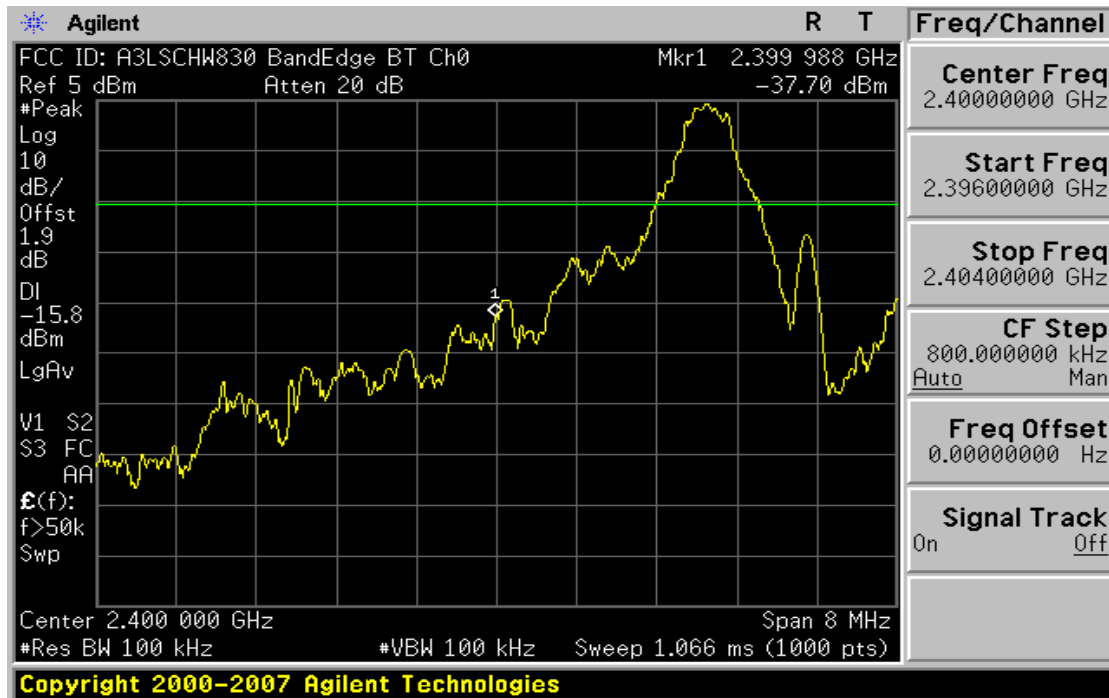
Plot 6-4. Band Edge Plot (Bluetooth – Ch. 0)
