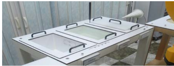
Figure 3.6 Modular Flat Phantom
