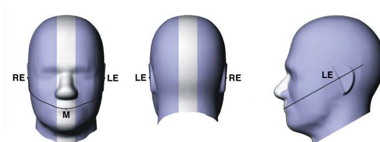
Figure 5.1 Front, back and side view of SAM
