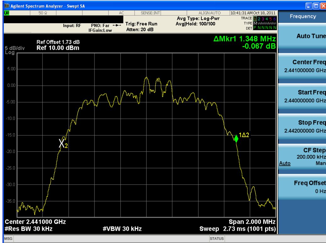
Plot 6-5. 20dB Bandwidth Plot (Bluetooth, 2Mbps – Ch. 39)
