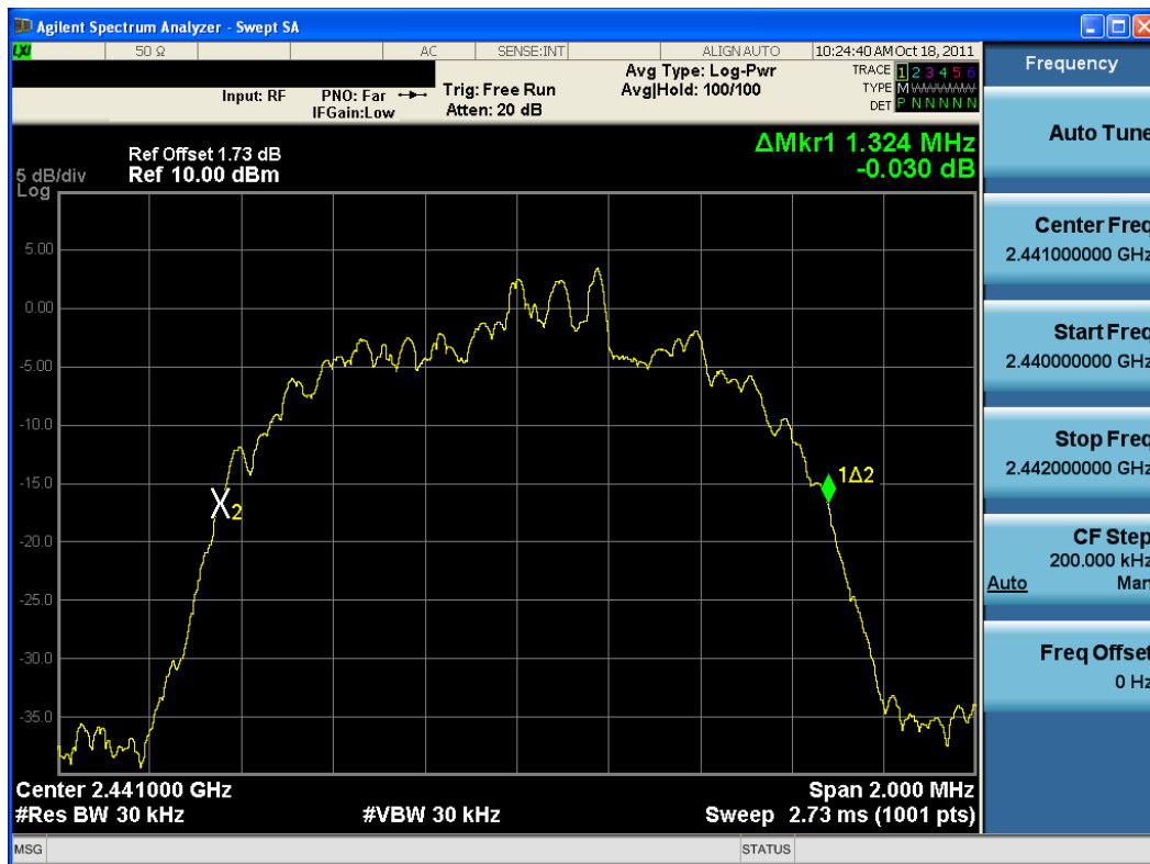
Plot 6-8. 20dB Bandwidth Plot (Bluetooth, 3Mbps – Ch. 39)
