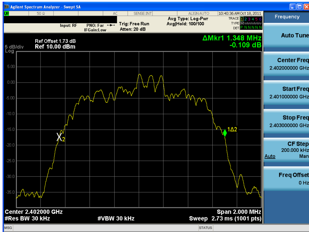
Plot 6-4. 20dB Bandwidth Plot (Bluetooth, 2Mbps – Ch. 0)
