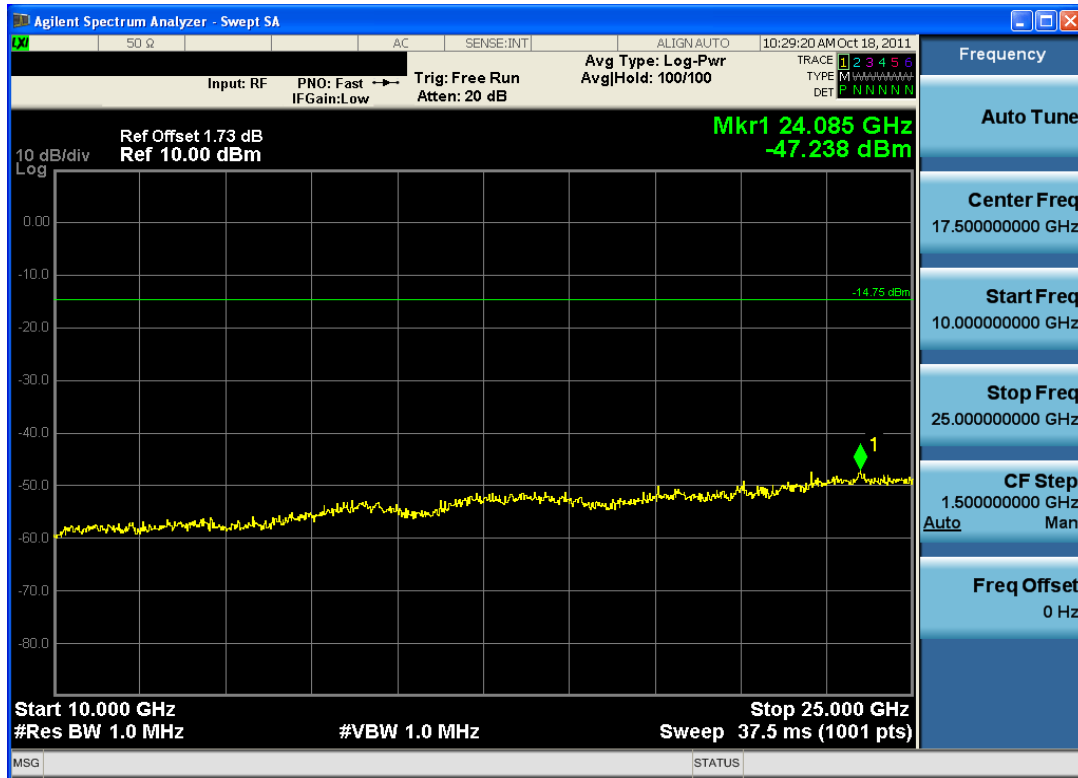
Plot 6-19. Conducted Spurious Plot (Bluetooth, 3Mbps – Ch. 39)
