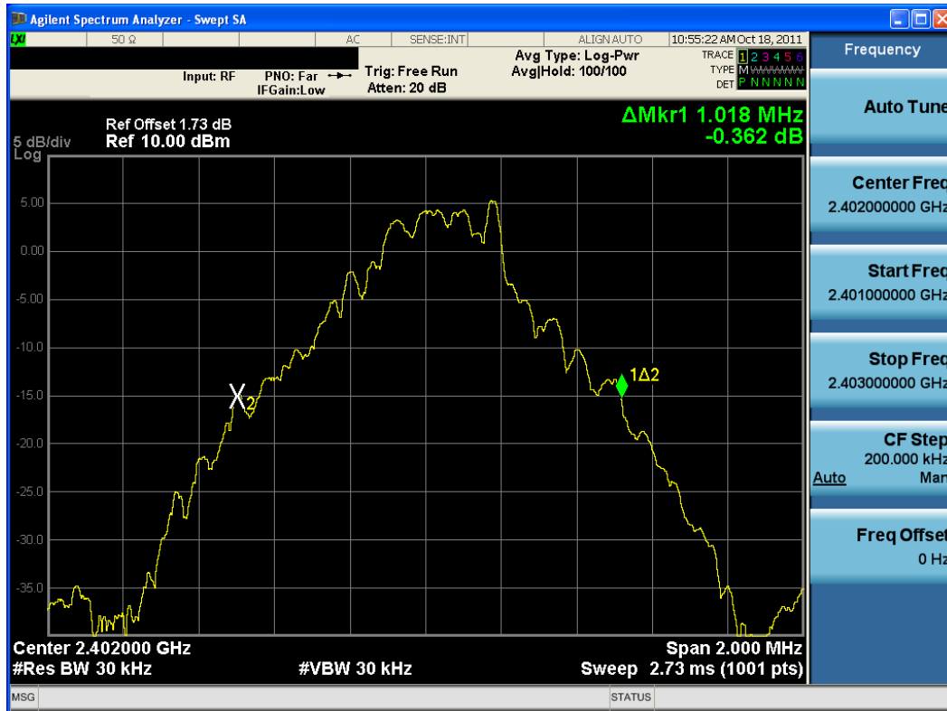
Plot 6-1. 20dB Bandwidth Plot (Bluetooth, 1Mbps – Ch. 0)
