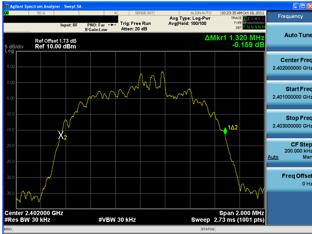
Plot 6-7. 20dB Bandwidth Plot (Bluetooth, 3Mbps – Ch. 0)
