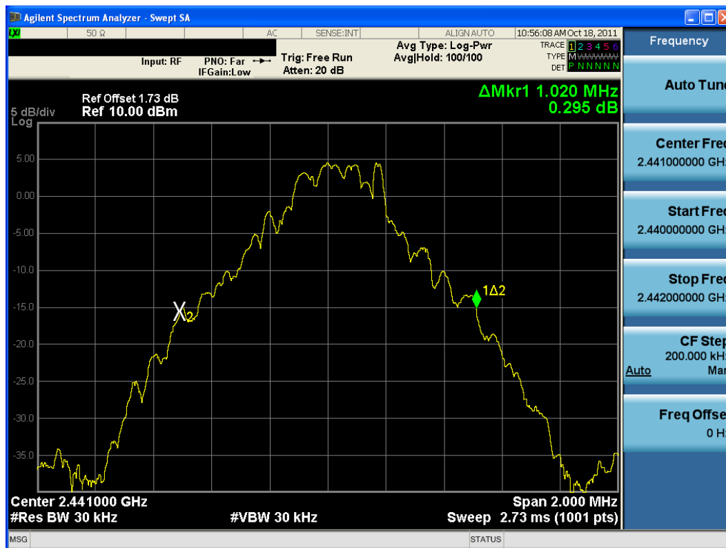
Plot 6-2. 20dB Bandwidth Plot (Bluetooth, 1Mbps – Ch. 39)
