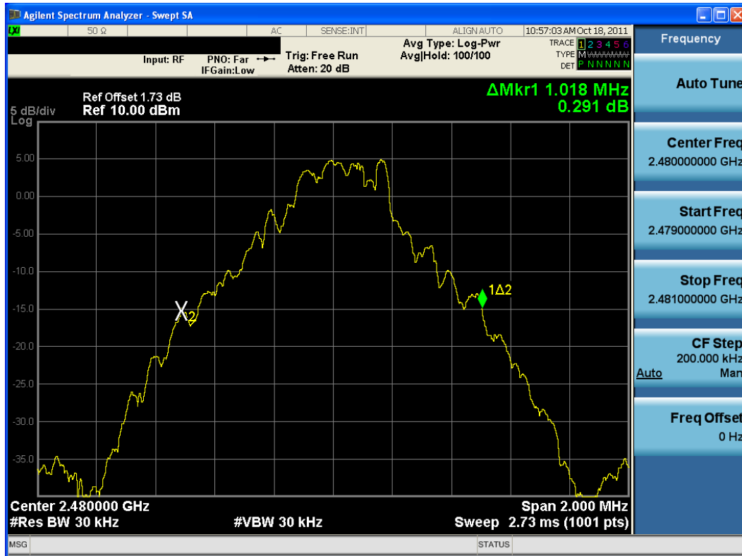
Plot 6-3. 20dB Bandwidth Plot (Bluetooth, 1Mbps – Ch. 78)
