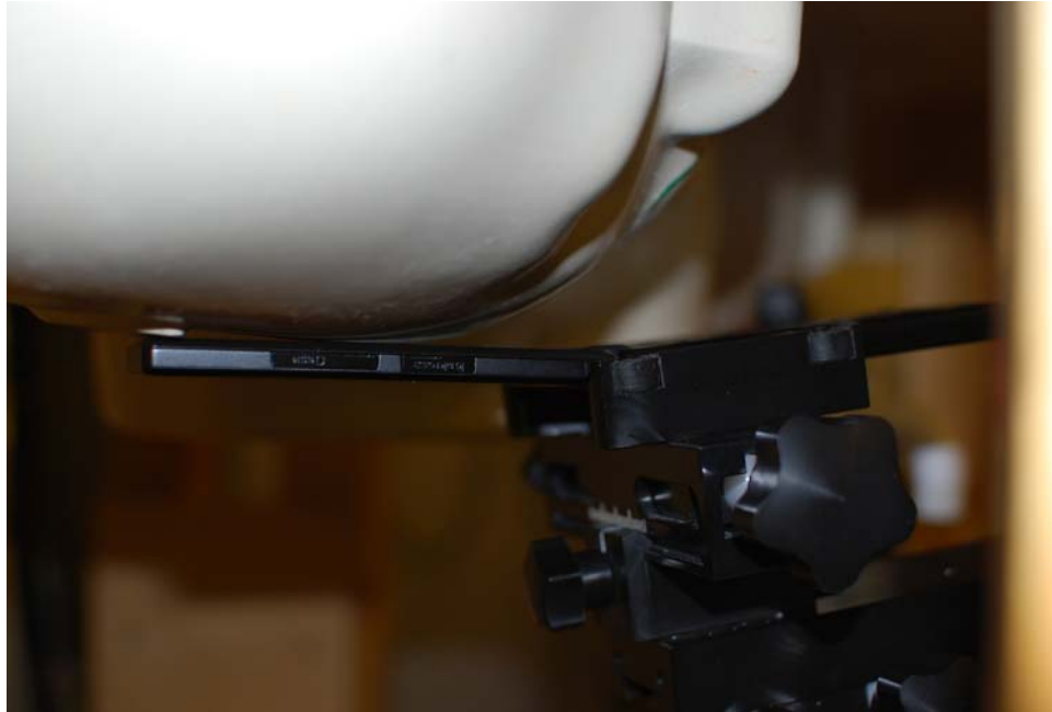
SAR Test Setup Photo 1 – Right Touch
