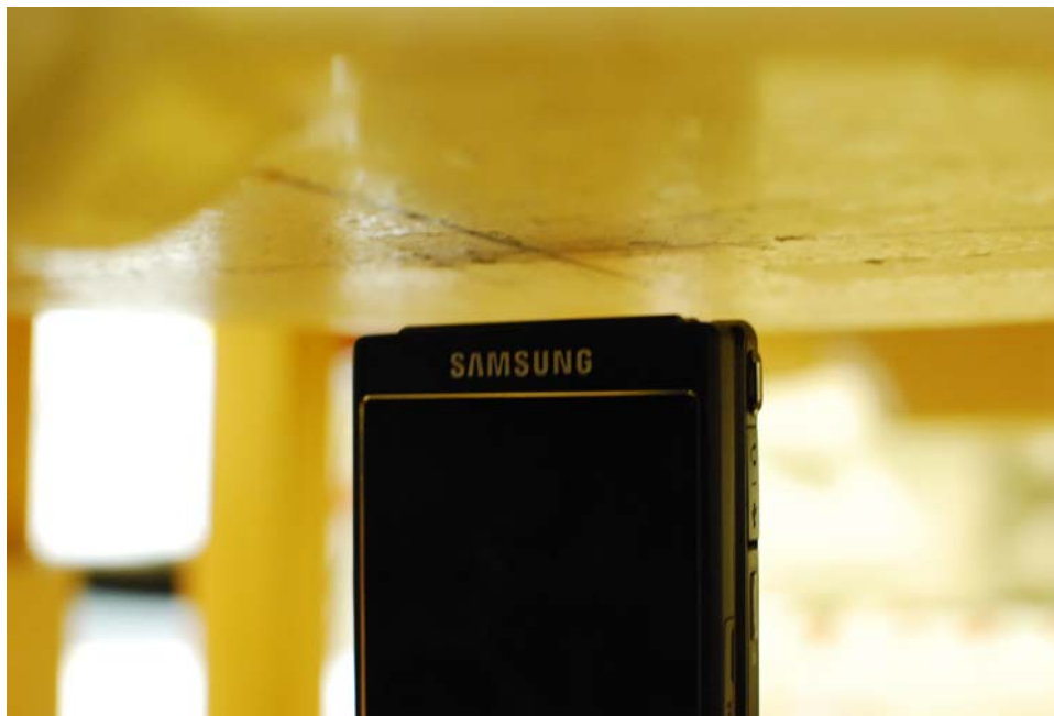
SAR Test Setup Photo 7 – Top at 1.0 cm
