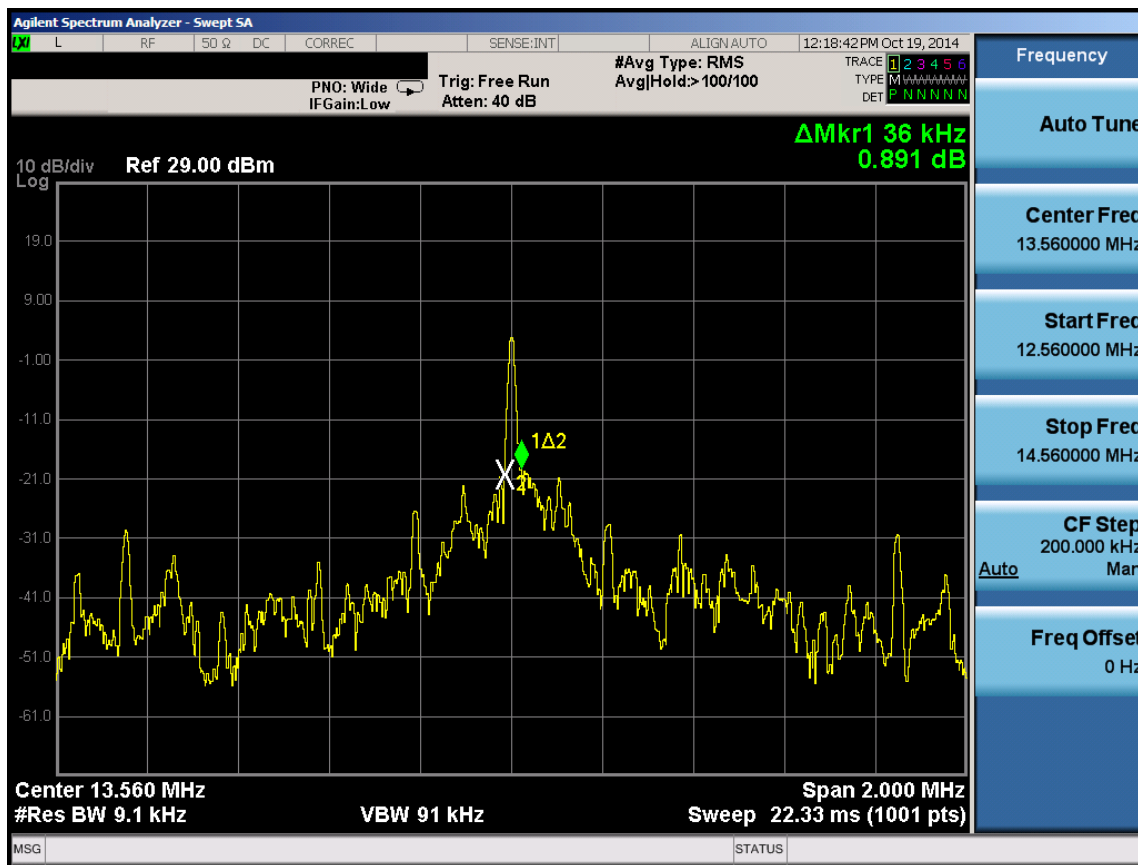
Figure 8-2. 20dB Bandwidth Plot
