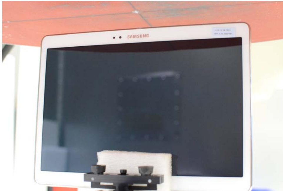
SAR Test Setup Photo 3: Top Edge at 2.0 cm
