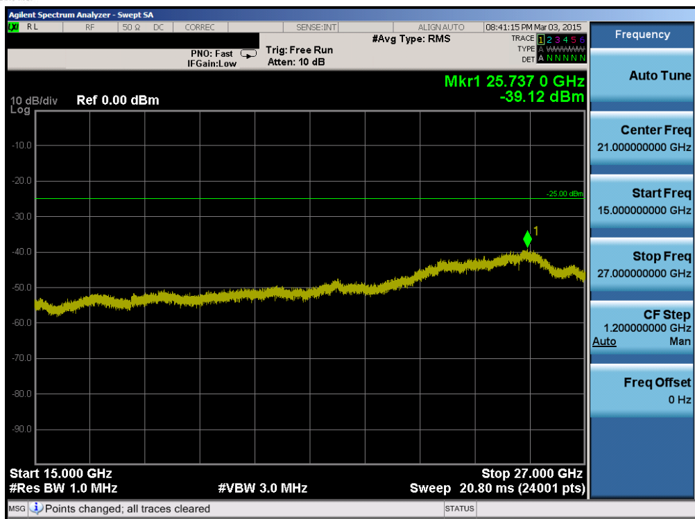
Plot 6-49. Conducted Spurious Plot (Band 41 – 20.0MHz QPSK – RB Size 1, RB Offset 0 – High Channel)
