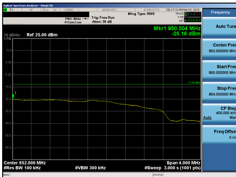
Plot 6-63. Upper Extended Band Edge Plot (Band 26 – 5.0MHz QPSK – RB Size 25)
