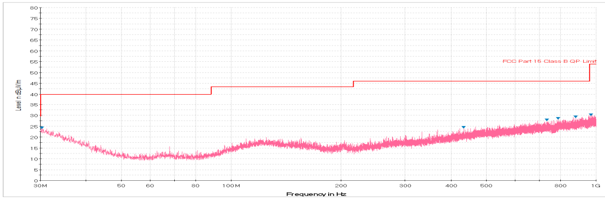
Plot 7-271. Radiated Spurious Plot below 1GHz (802.11a – U3 Ch. 157, Ant. Pol. V)
