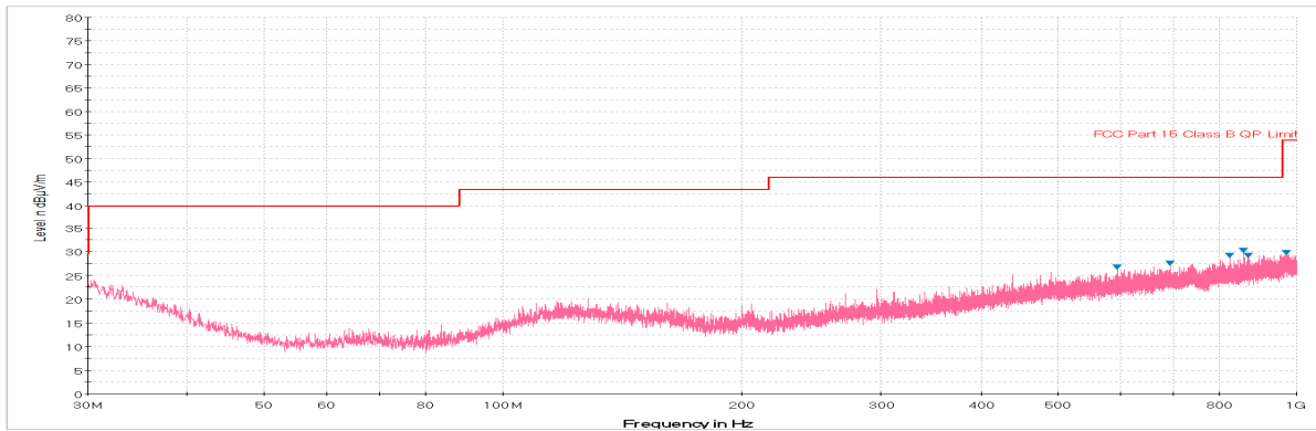
Plot 7-95. Radiated Spurious Plot below 1GHz (Pol. H)
