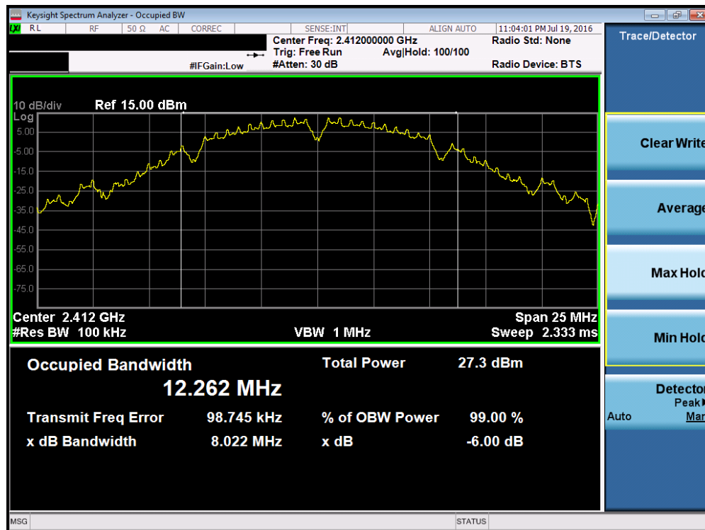
Plot 7-10. 6dB Bandwidth Plot (802.11b – Ch. 1)
