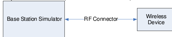
Figure 9-4 Power Measurement Setup
