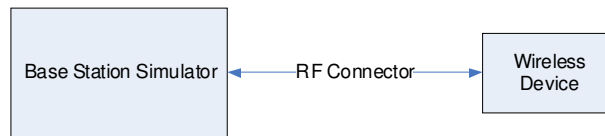
Figure 9-2 Power Measurement Setup
