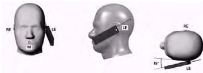
Figure 6-2 Front, Side and Top View of Ear/15° Tilt Position
