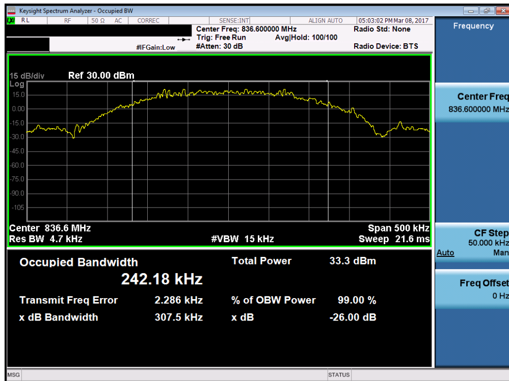
Plot 7-2. Occupied Bandwidth Plot (EDGE850 Mode – Ch. 190)
