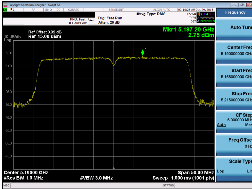
Plot 7-85. Power Spectral Density Plot (40MHz BW 802.11n (UNII Band 1) – Ch. 38)
