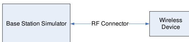
Figure 9-4 Power Measurement Setup
