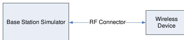
Figure 9-1 Power Measurement Setup
