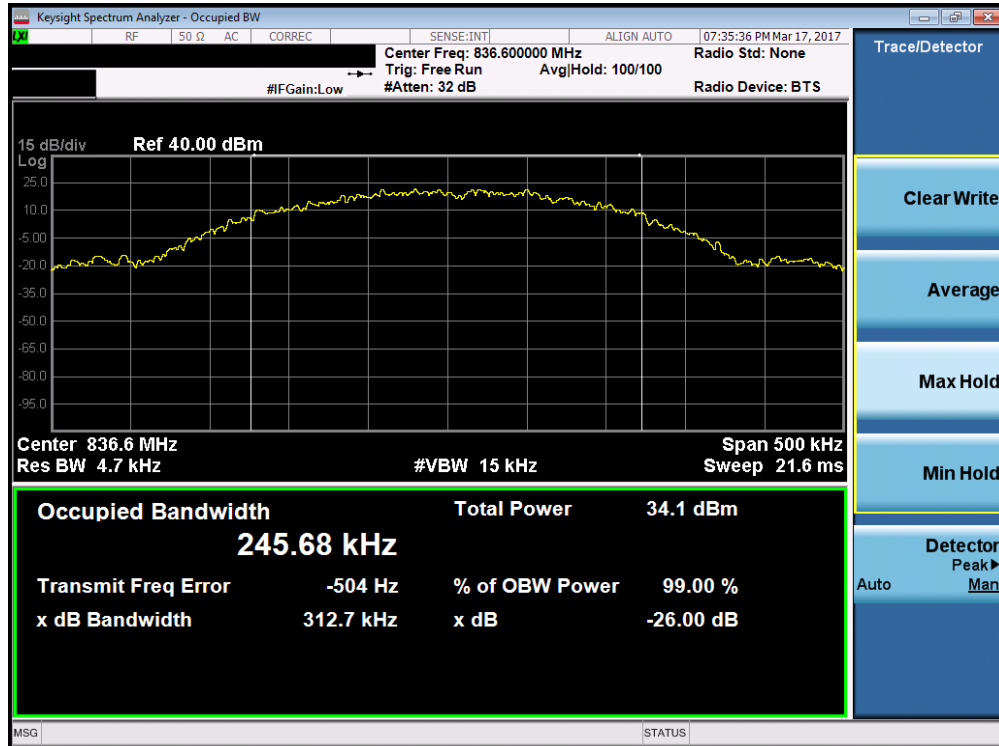
Plot 7-1. Occupied Bandwidth Plot (Cellular GPRS Mode – Ch. 190)
