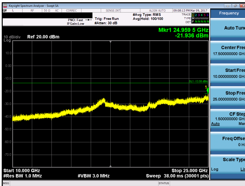
Plot 7-28. Conducted Spurious Plot (Bluetooth (LE) – 1Mbps, Ch. 39)
