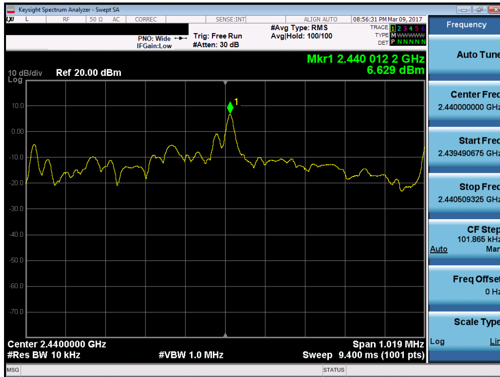
Plot 7-14. Power Spectral Density Plot (Bluetooth (LE) – 1Mbps, Ch. 19)
