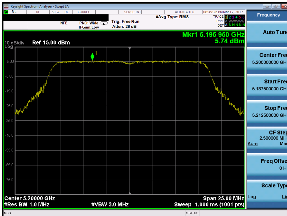
Plot 7-119. Power Spectral Density Plot (802.11a (UNII Band 1) – Ch. 40)
