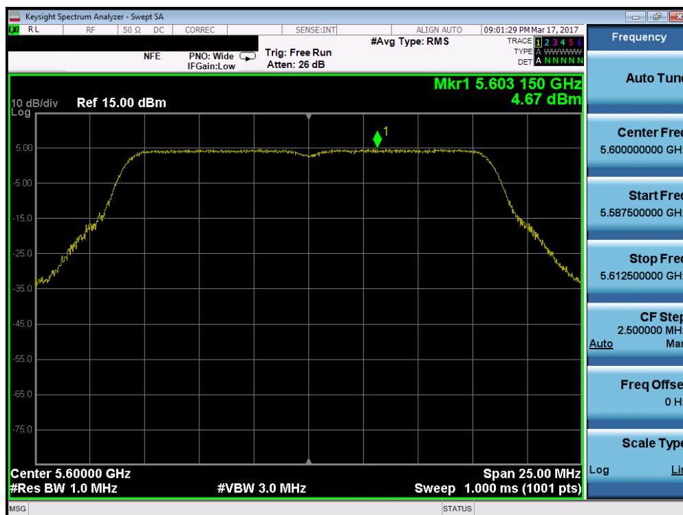
Plot 7-137. Power Spectral Density Plot (802.11a (UNII Band 2C) – Ch. 120)
