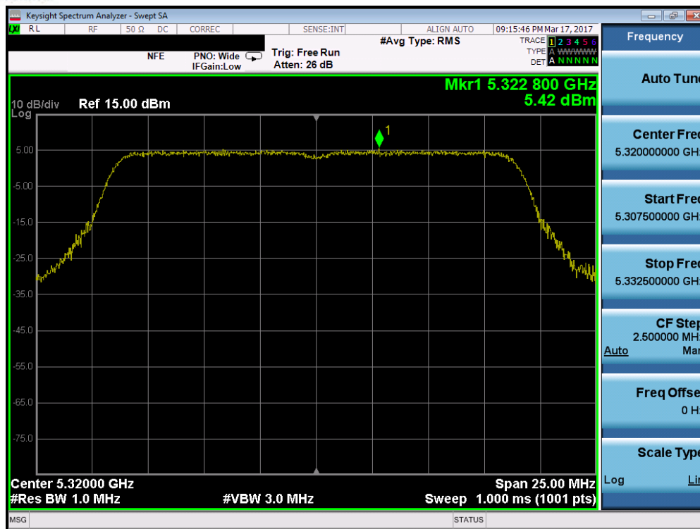
Plot 7-132. Power Spectral Density Plot (20MHz BW 802.11n (UNII Band 2A) – Ch. 64)
