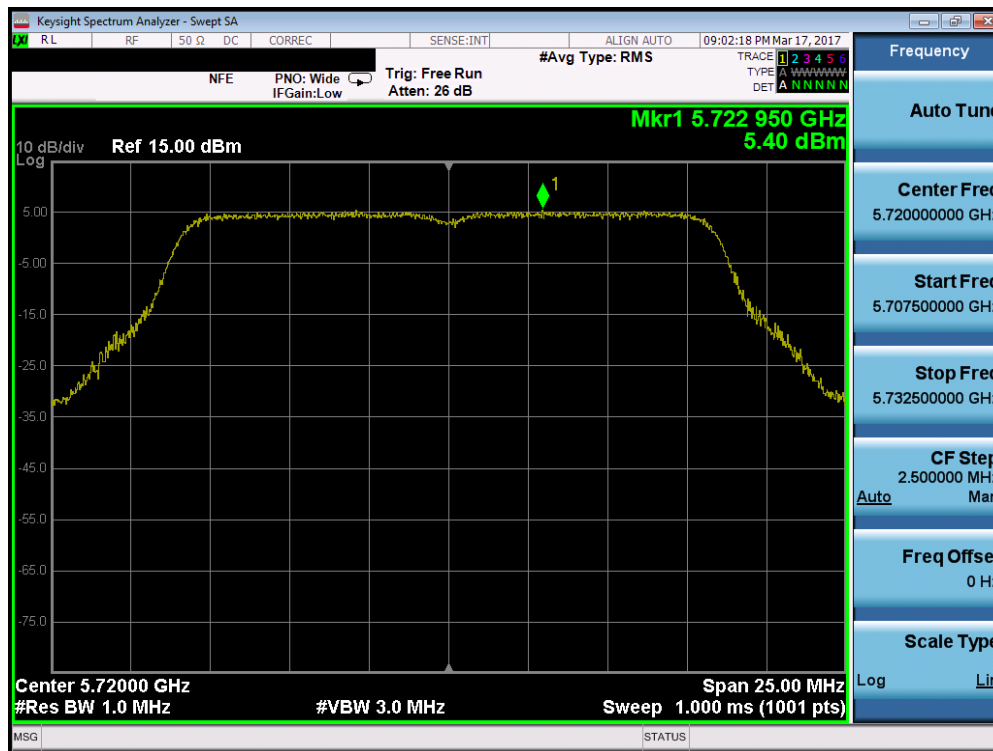
Plot 7-138. Power Spectral Density Plot (802.11a (UNII Band 2C) – Ch. 144)
