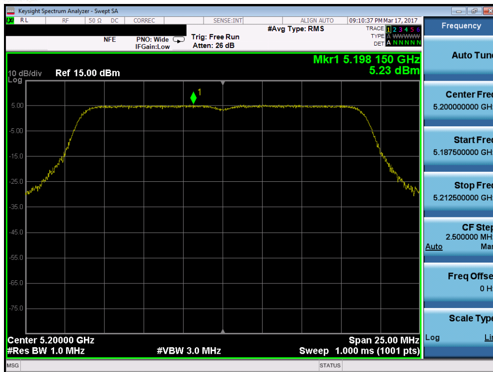
Plot 7-122. Power Spectral Density Plot (20MHz BW 802.11n (UNII Band 1) – Ch. 40)
