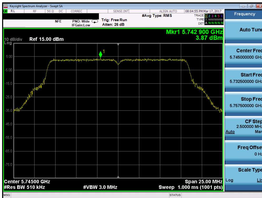
Plot 7-109. Power Spectral Density Plot (802.11a (UNII Band 3) – Ch. 149)
