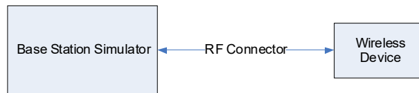
Figure 9-1 Power Measurement Setup
