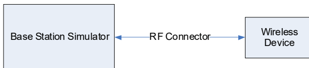
Figure 9-3 Power Measurement Setup
