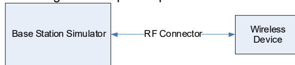
Figure 9-2 Power Measurement Setup
