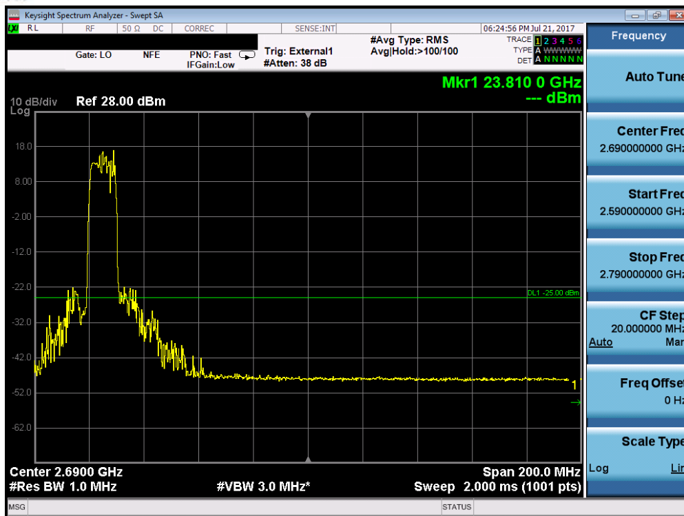
Plot 7-285. PC2 Upper ACP Plot (Band 38 – 10.0MHz QPSK – RB Size 50)
