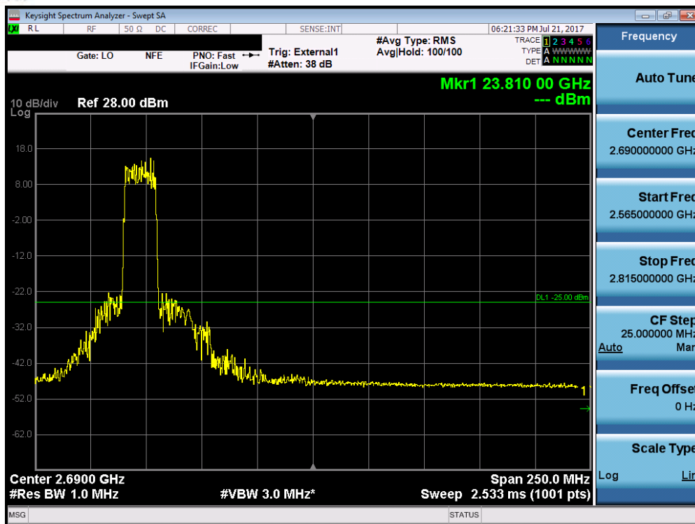
Plot 7-285. PC2 Upper ACP Plot (Band 38 – 15.0MHz QPSK – RB Size 75)
