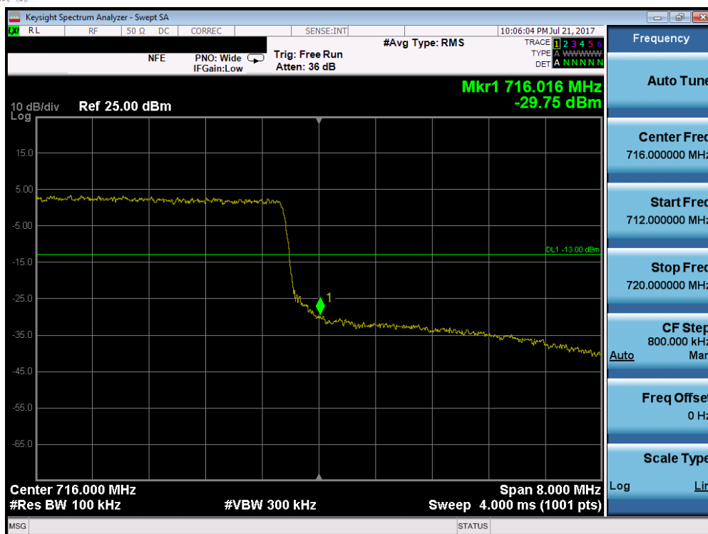
Plot 7-100. Upper Band Edge Plot (Band 17 – 10.0MHz QPSK – RB Size 50)
