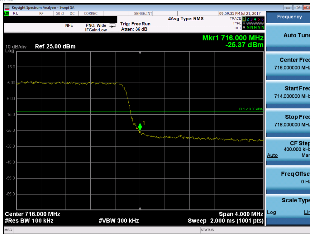
Plot 7-98. Upper Band Edge Plot (Band 17 – 5.0MHz QPSK – RB Size 50)
