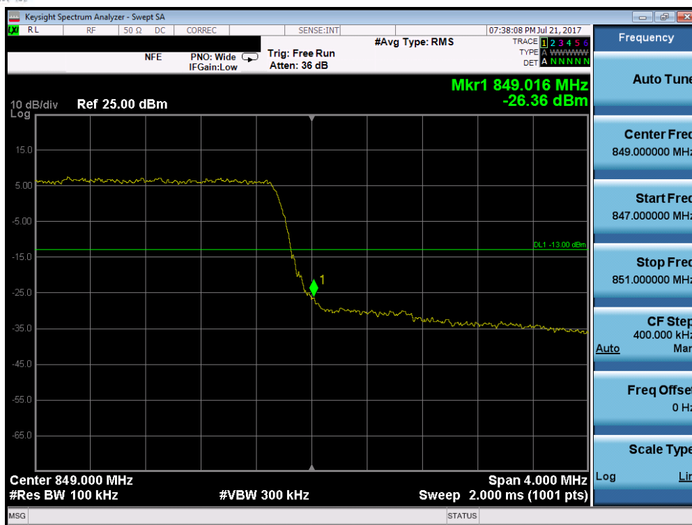
Plot 7-114. Upper Band Edge Plot (Band 5/26 – 5.0MHz QPSK – RB Size 25)
