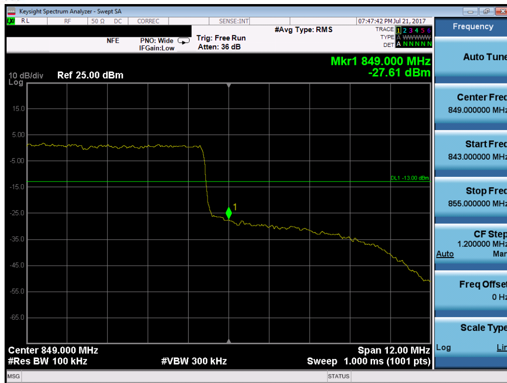
Plot 7-118. Upper Band Edge Plot (Band 26 – 15.0MHz QPSK – RB Size 75)
