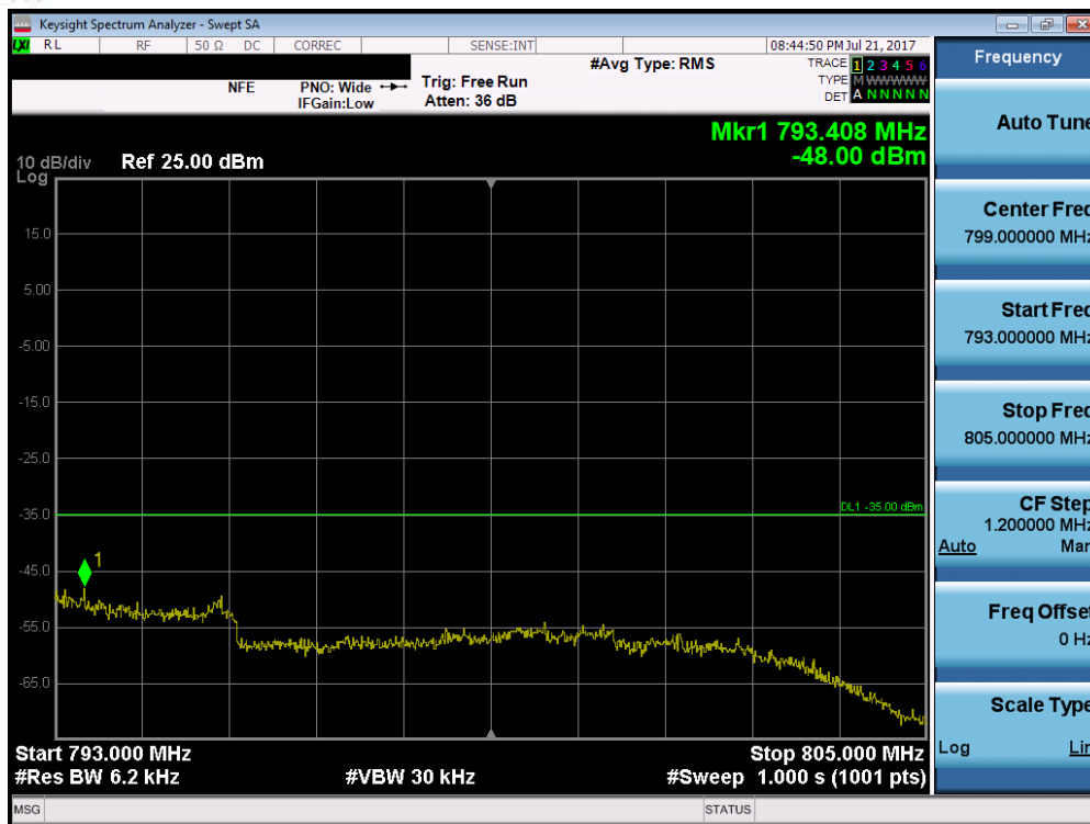
Plot 7-108. Upper Emission Mask Edge Plot (Band 13 – 10.0MHz QPSK – RB Size 50)
