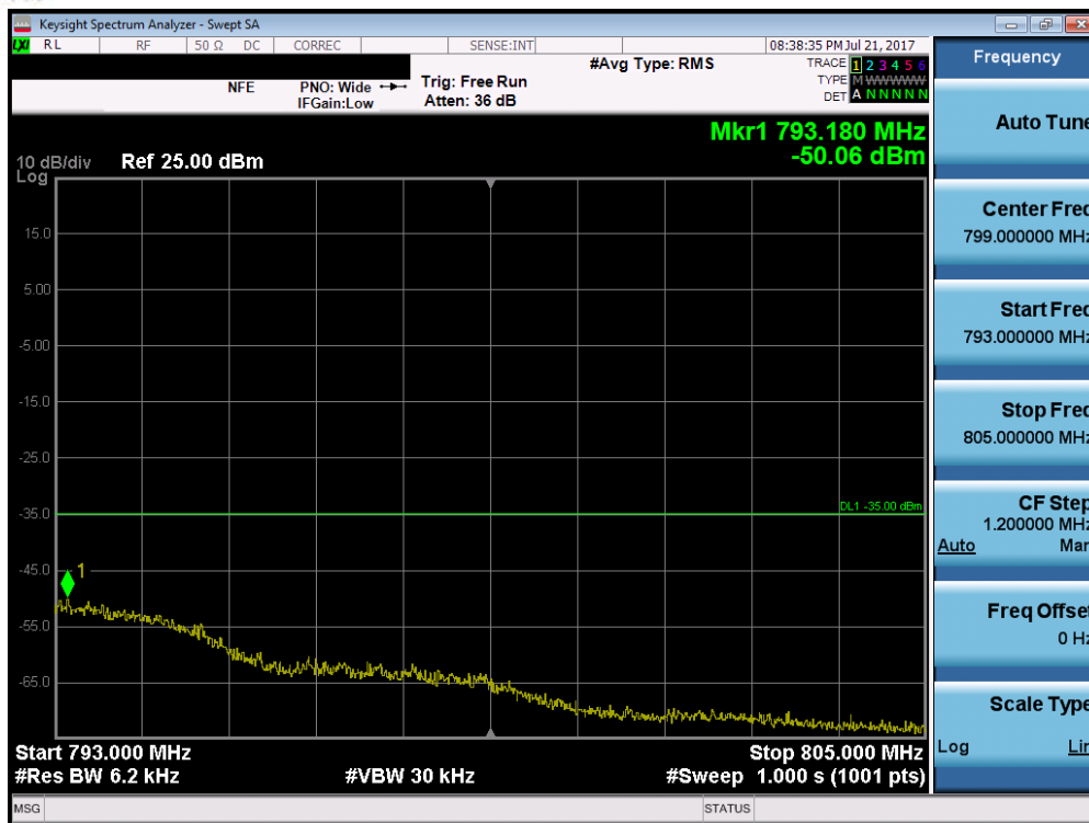
Plot 7-104. Upper Emission Mask Edge Plot (Band 13 - 5.0MHz QPSK - RB Size 25)
