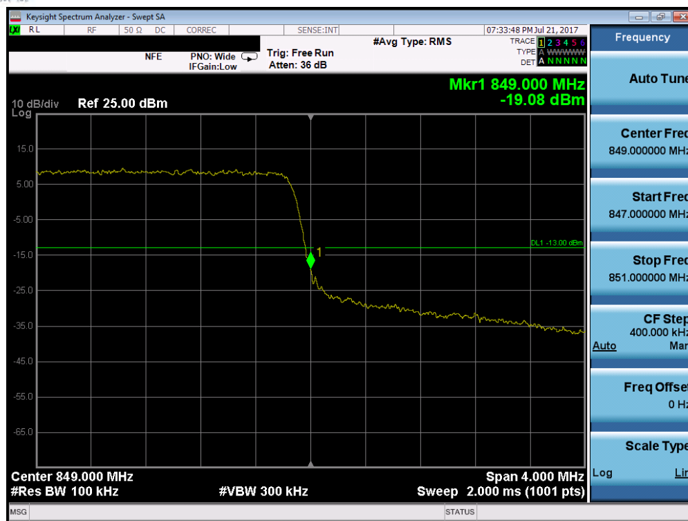
Plot 7-112. Upper Band Edge Plot (Band 5/26 – 3.0MHz QPSK – RB Size 15)
