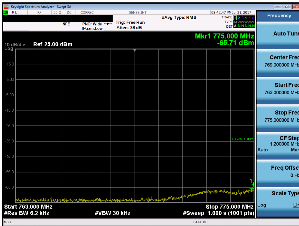
Plot 7-106. Lower Emission Mask Edge Plot (Band 13 – 10.0MHz QPSK – RB Size 50)
