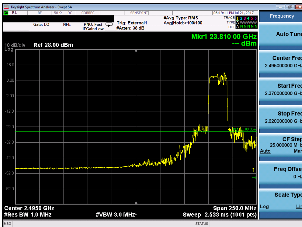
Plot 7-285. PC2 Lower ACP Plot (Band 38 – 20.0MHz QPSK – RB Size 100)
