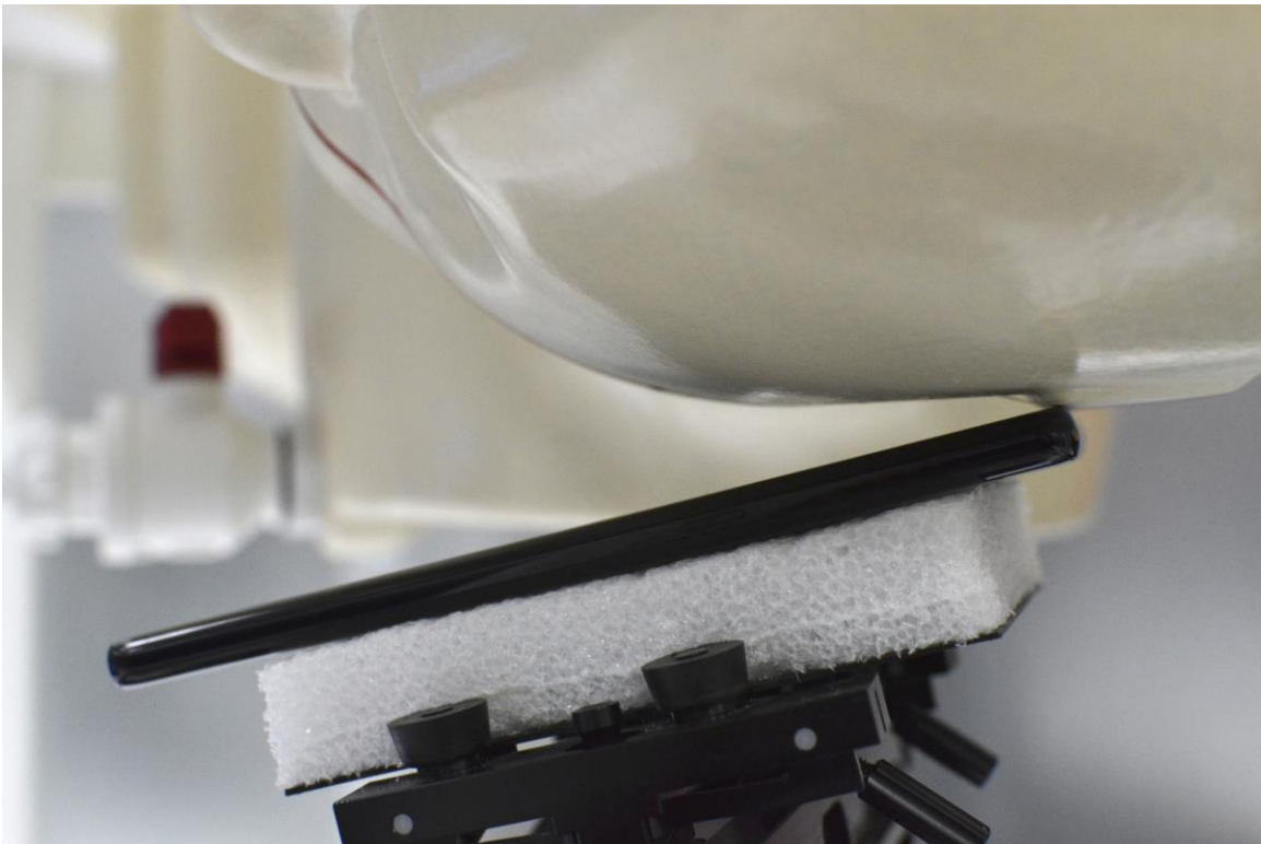
SAR Test Setup Photo 4 – Left Tilt
