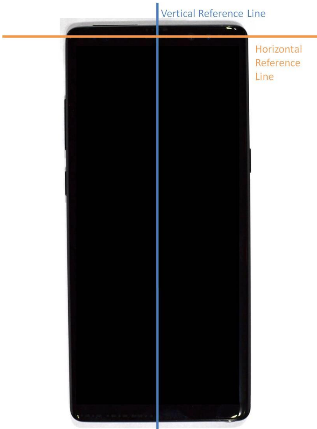
SAR Test Setup Photo 17 – Horizontal and Vertical Reference Lines
