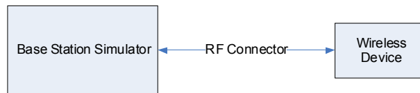
Figure 9-1 Power Measurement Setup
