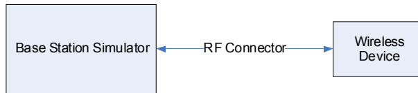
Figure 9-1 Power Measurement Setup
