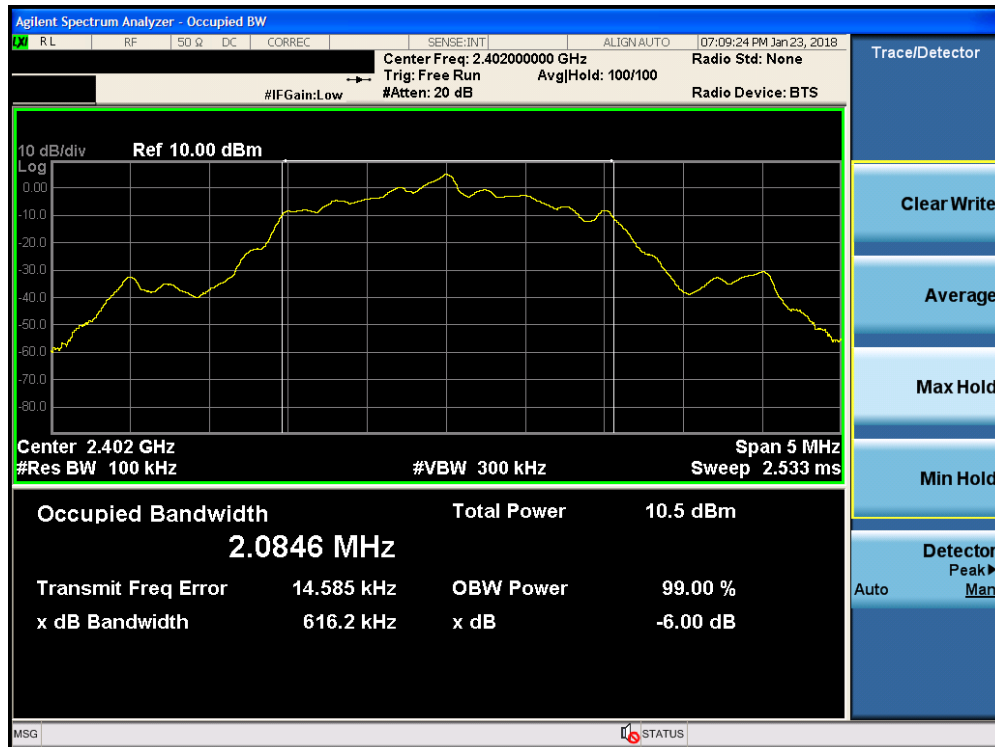
Plot 7-4. 6dB Bandwidth Plot (Bluetooth (LE), 2Mbps – Ch. 0)
