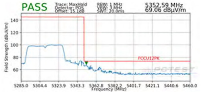
Plot 7-222. Radiated Band Edge Plot (Peak – WCP)
