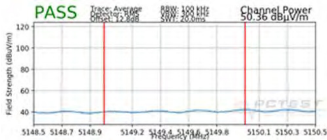
Plot 7-241. Radiated Lower Band Edge Plot (Average – UNII Band 1)
